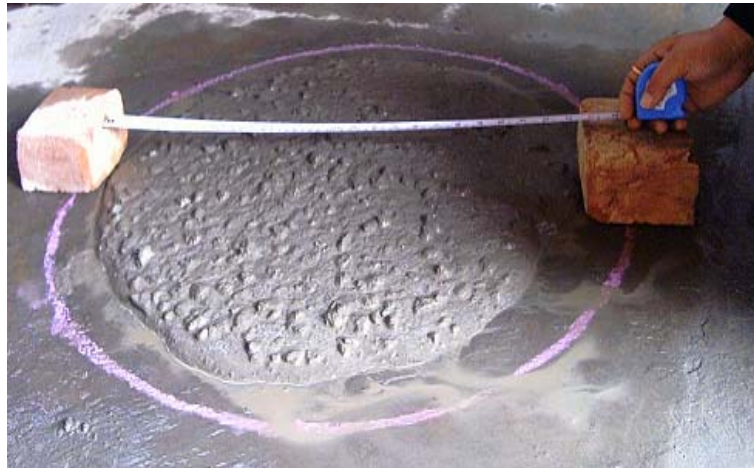
Figure 1. Slump Flow Test
