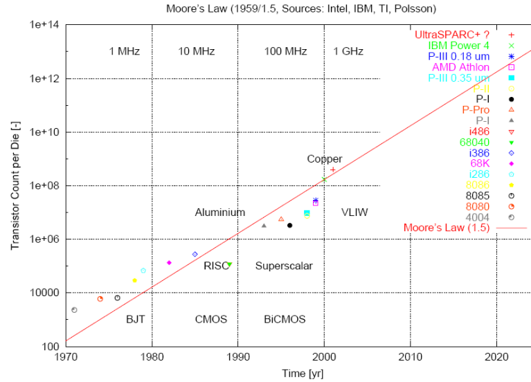
Figure 1. Moore's Law for microprocessor transistor counts assuming a starting point of 1960 and doubling time of 18 months.
