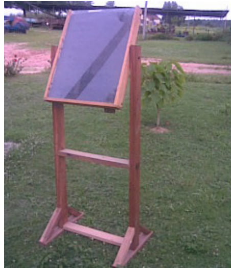
Figure 5. The collector tilted to receive insolation
