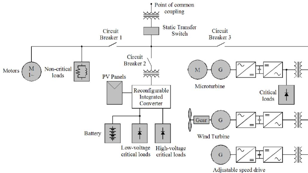
**Figure 3.** Configuration of a typical AC micro-grid
