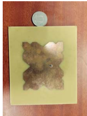
Figure 8. Fabricated Prototype of Proposed Antenna
