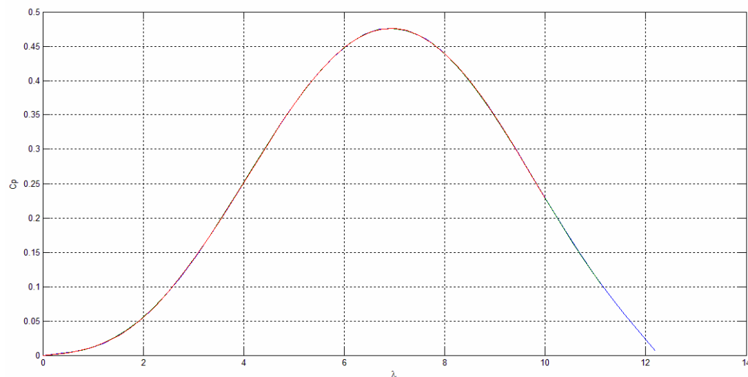
Figure 4. Power coefficients versus rotational speed in different cases of wind speed
