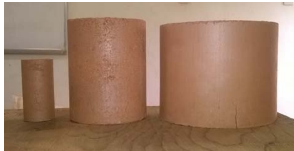
Figure 3. Soil sample for split former mould, proctor mould and California bearing ratio mould used for the study
