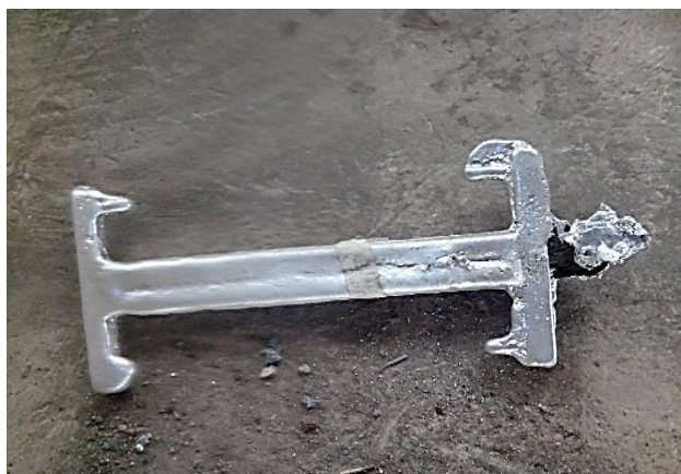
Figure 6 (a). Incomplete filling of the mould at 680^{\circ}\text{C} (Low fluidity)
